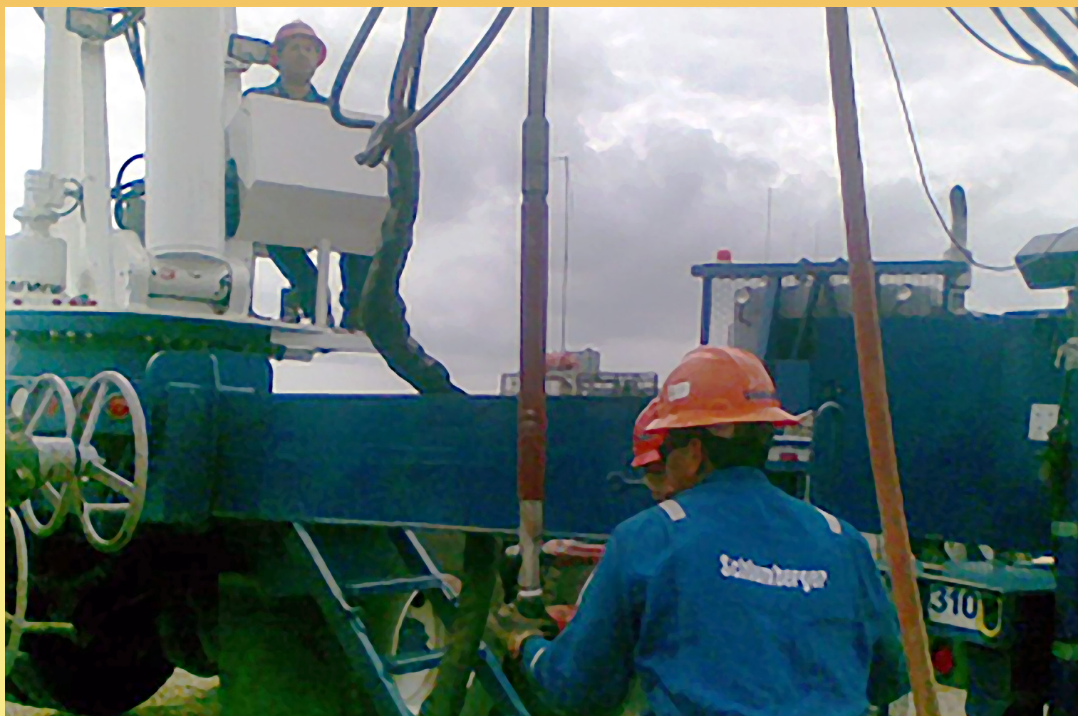
Figure 2. TF with BN mandrel at the end.
