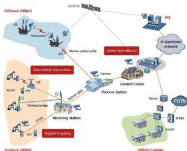
Figure 1 Oil and gas digital production solution network
